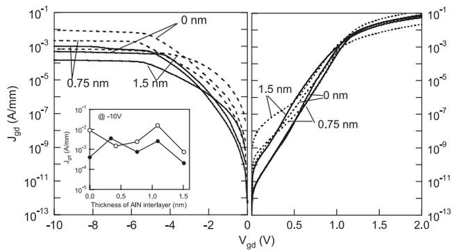
**Fig. 6** Gate leakage current of the samples with 0-, 0.75-, and 1.5-nm-thick AlN interlayers. Dotted lines and solid lines show the current of InAlN/GaN and InAlN/AlGaIn/GaN, respectively. Inset shows the reverse leakage current at  $V_{gd} = -10 \text{ V}$  as a function of the AlN interlayer thickness. Open circles and closed circles show the data for InAlN/GaN and InAlN/AlGaIn/GaN, respectively.
