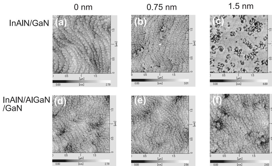
**Fig. 2** AFM images of surface morphologies of InAlN/GaN and InAlN/AlGaIn/GaN heterostructures with 0-, 0.75-, and 1.5-nm-thick AlN interlayers.
