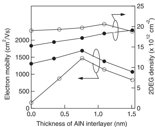
**Fig. 3** Electron mobility and 2DEG density of InAlN/GaN (open circles) and InAlN/AlGaIn/GaN (closed circles) as a function of AlN interlayer thickness.
