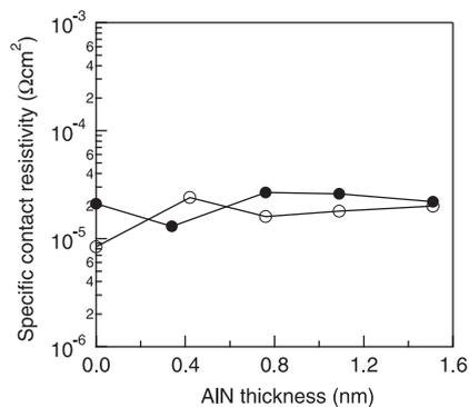
**Fig. 4** Specific contact resistivity of InAlN/GaN (open circles) and InAlN/AlGaIn/GaN (closed circles) as a function of AlN interlayer thickness.
