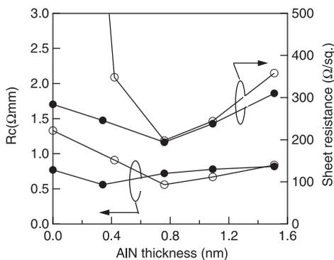
**Fig. 5** Contact resistance and sheet resistance of InAlN/GaN (open circles) and InAlN/AlGaIn/GaN (closed circles) as a function of AlN interlayer thickness.
