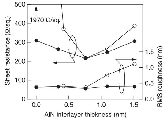
**Fig. 1** Sheet resistance and rms roughness of the surface as a function of AlN interlayer thickness. Open and closed circles show the data for InAlN/GaN and InAlN/AlGaIn/GaN, respectively.
