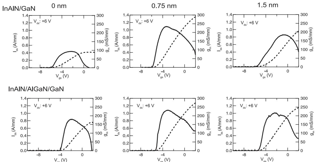
**Fig. 7** Transfer characteristics of InAlN/GaN and InAlN/AlGaIn/GaN heterostructures FETs with 0-, 0.75-, and 1.5-nm-thick AlN interlayers.
