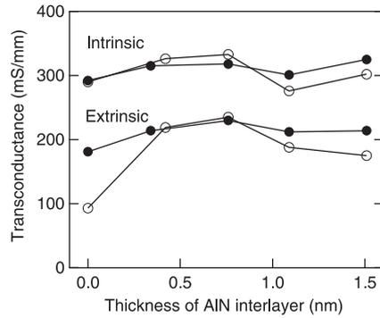
**Fig. 8** Intrinsic and extrinsic maximum transconductance as a function of AlN interlayer thickness. Open circles and closed circles show the data for InAlN/GaN and InAlN/AlGaIn/GaN, respectively.
